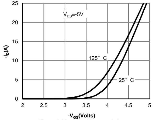
Figure 2: Transfer Characteristics
