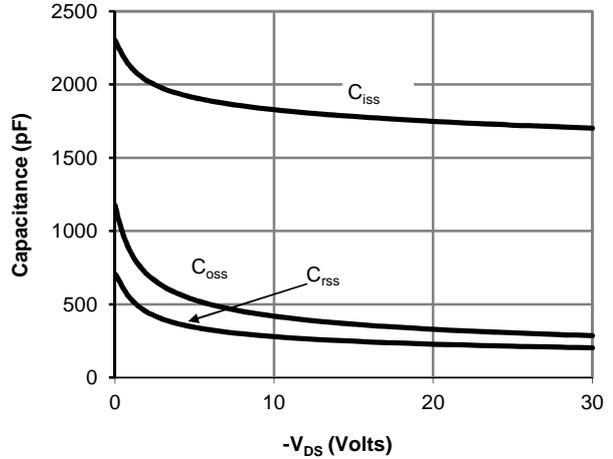
Figure 8: Capacitance Characteristics
